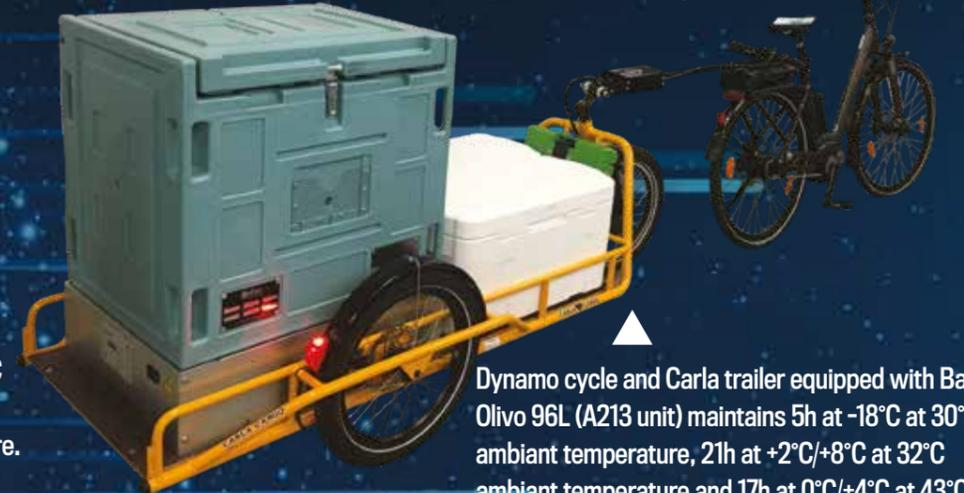
▲ Dynamo cycle and Carla trailer equipped with Bac Olivo 96L (A213 unit) maintains 5h at -18°C at 30°C ambient temperature, 21h at +2°C/+8°C at 32°C ambient temperature and 17h at 0°C/+4°C at 43°C ambient temperature.
