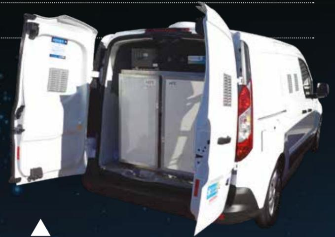
▲ Renault Kangoo equipped with a dual temperature container 2x200L (A413 unit); maintains 19h at +2°C/+8°C at 32°C ambient temperature and 21h at +15°C/+25°C at -10°C ambient temperature.
