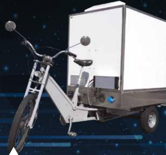
▲ Lovelo, electrically assisted tricycle equipped with a specific 720L container (A413 unit); maintains 12h at 0°C/+4°C at ambient temperature of 30°C.
