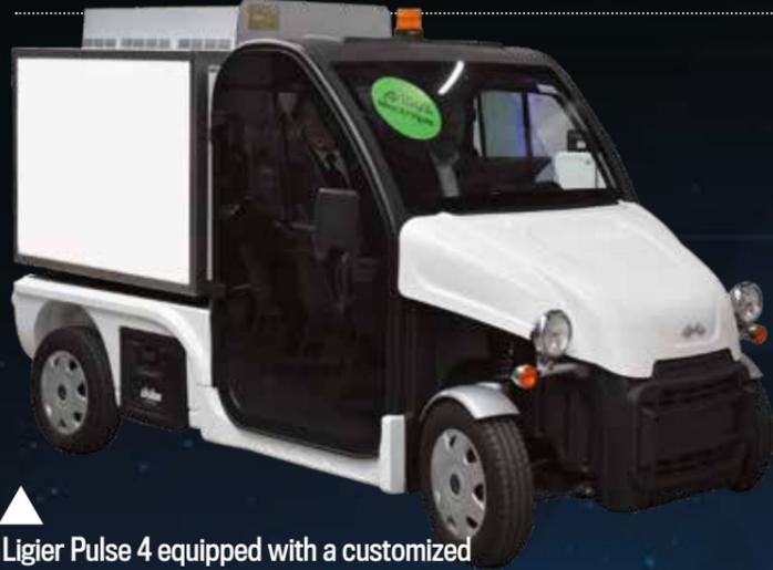
▲ Ligier Pulse 4 equipped with a customized 1200L container (A420 unit); maintains 0°C/+4°C up to 19h with an ambient temperature at 32°C.
